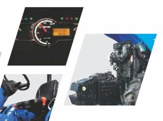
3 CYLINDER TURBOCHARGED WITH INTERCOOLER
