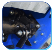
ANTI WRAPPING GUARD ON ROLLER & ROTOR
