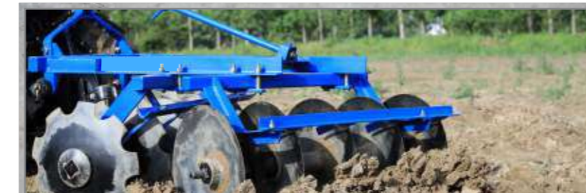
Useful for open field for superficial ploughing for shattering of clods, preparing seed bed, burial of organic substance and remains of cut of crop
