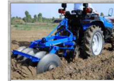
Used for chopping up unwanted weeds or crop residue
