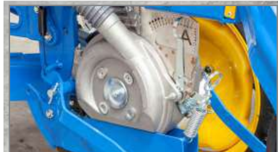
Precise metering device to sow seeds of different sizes such as maize, peas, sunflower, soybean, etc.
